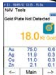
The Niton DXL's patent-pending AuDIT feature instantly warns you of the probability of gold plated material
