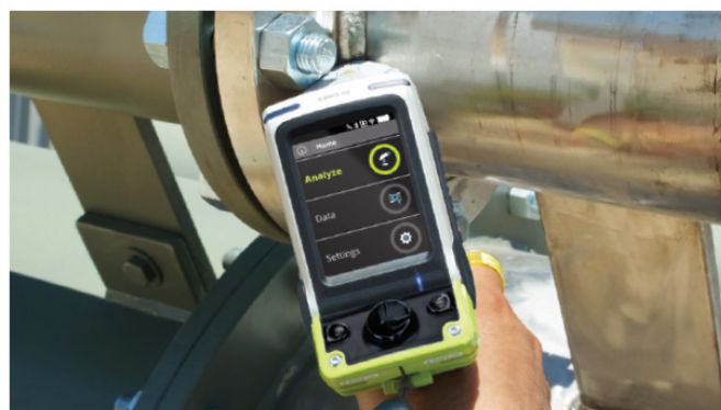
The Niton XL5 Plus in use, analysing a tight weld in an oil refinery.
