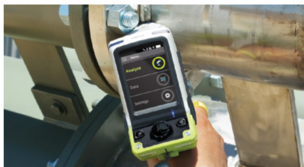
The Niton XL5 in use, analysing a tight weld in an oil refinery.
